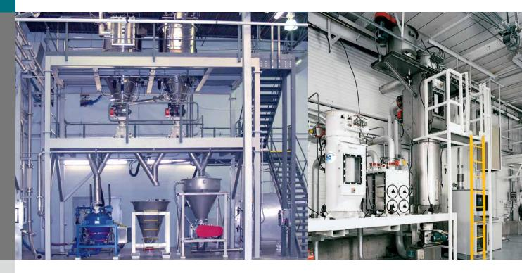
Unique to the filtration industry, the Schenck Process TestCenter includes a Particle Emissions Test (PET) system that records and graphs air flow and velocity, air-to-cloth ratios, pressure differentials, inlet loading and outlet mass emissions. The system also accurately predicts PM2.5 emissions and provides the necessary information to design the most ideal solution based on the customer's requirements and application.
