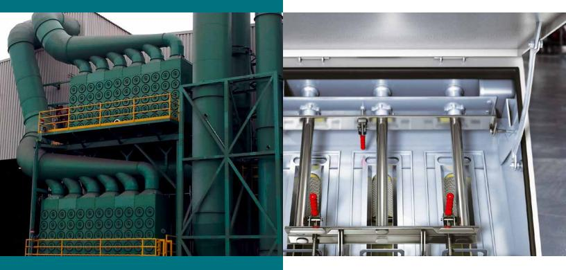
The Mac2Flo® provides cost-effective filtration of the finest submicron dusts. The unit operates using the downflow principle, which guarantees effective settling of the fine, light dusts with low terminal settling velocities. As each filter cartridge can contain up to 254 ft² of media, large filtration potential can be housed within a relatively compact housing.
